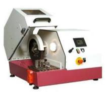
wheels are used. Adding to this, effective sample cooling is a key factor in producing high quality burn-free cuts.
