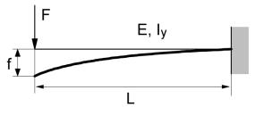
Fig. 1.2 cantilever beam
