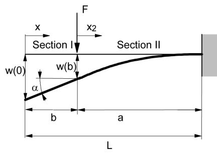
Fig. 1.3 Elastic line of a cantilever beam
