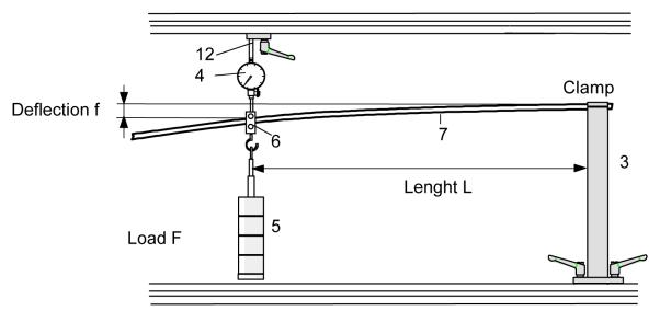
Fig. 1.2 experiment setup
