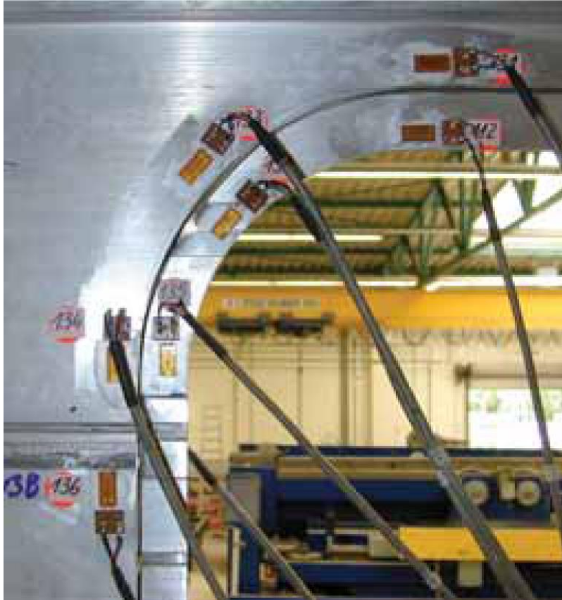
Strain gages in railway engineering Experimental stress analysis on a railway car
