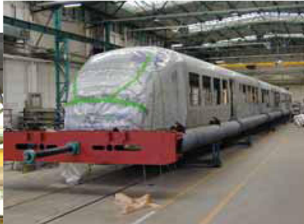
Strain gages in railway engineering Experimental stress analysis on a railway car
