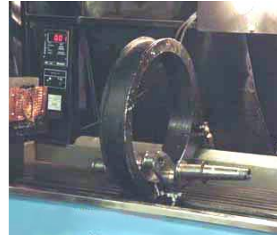
Coil on Wet Horizontal Inspection Unit
