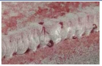
Non-relevant weld geometry indications
