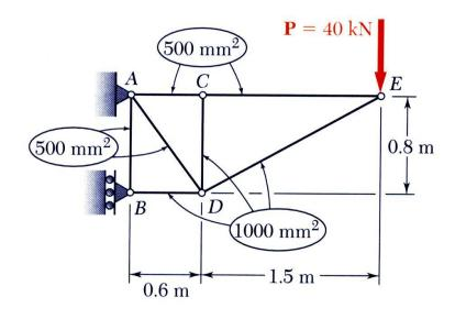
Members of the truss shown consist of sections of aluminum pipe with the cross-sectional areas indicated. Using E = 73 GPa, determine the vertical deflection of the point *E* caused by the load P.
