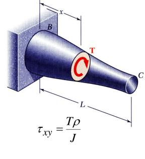
• For a shaft subjected to a torsional load,
