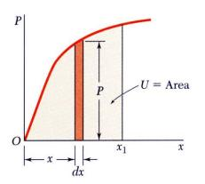
• The *elementary work* done by the load P as the rod elongates by a small dx is
