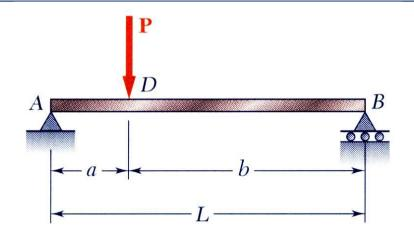
Taking into account only the normal stresses due to bending, determine the strain energy of the beam for the loading shown. SOLUTION:
