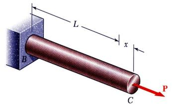
• Previously, we found the strain energy by integrating the energy density over the volume. For a uniform rod,
