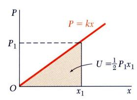
• In the case of a linear elastic deformation,
