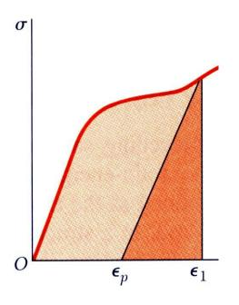
To eliminate the effects of size, evaluate the strainenergy per unit volume,
